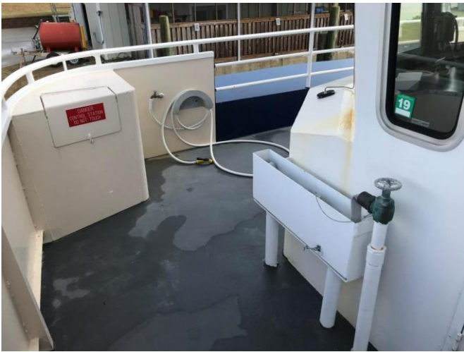
Photo # 33 – Port side bridge deck with wing station and bridge deck fire station
