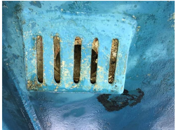
Photo # 6 – Port side main engine sea chest fouling
