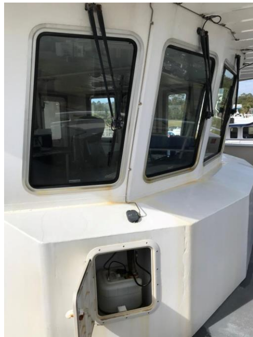
Photo # 32 – Forward bulkhead of pilot house with windshield wipers and wash system
