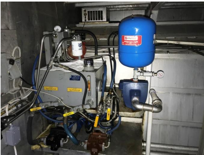
Photo # 57 – Comp. # 6S – Hydraulic steering system & Fresh water pressure set & de-humidifier in the background
