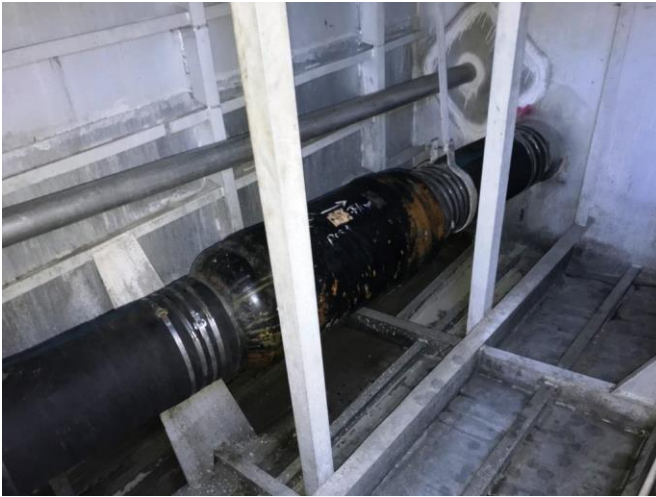
Photo # 47 – Comp. # 5 – Port side M/E exhaust muffler
