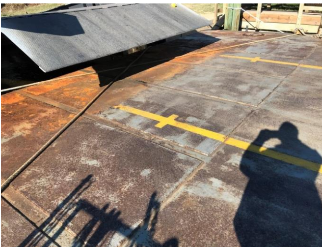
Photo # 1 – Main Deck at bow showing wear plates
