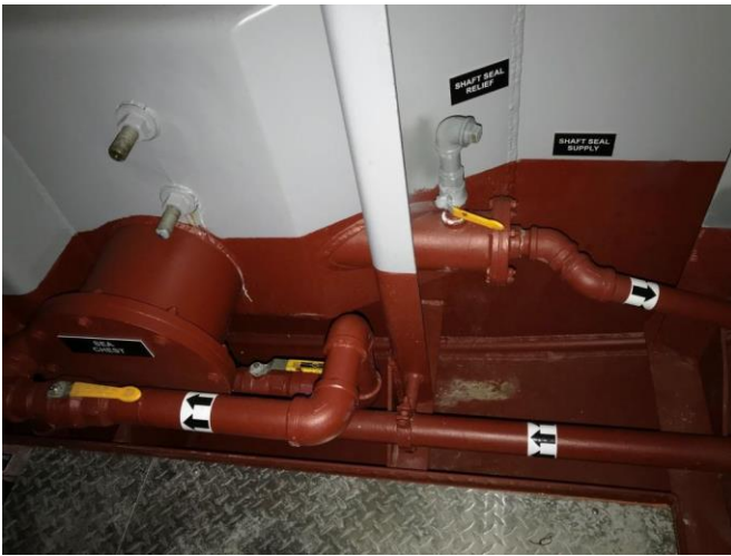
Photo # 29 – Sea suction & keel cooler connection
