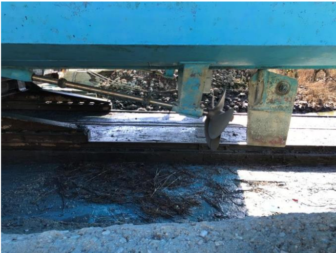
Photo # 5 – Port side tail shaft, prop, and rudder
