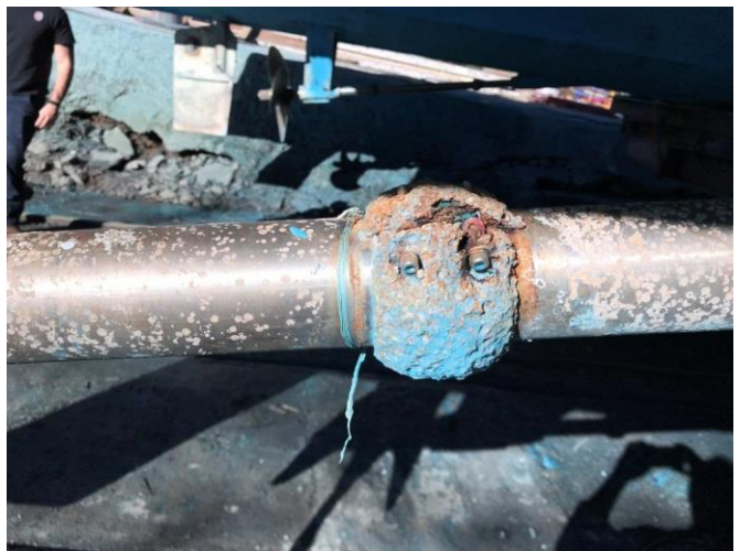
Photo # 14 – Wasted anode condition on propeller shaft
