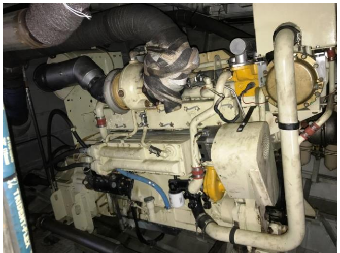
Photo # 42 – Comp. # 4 – Stbd. side main engine – 640 HP
