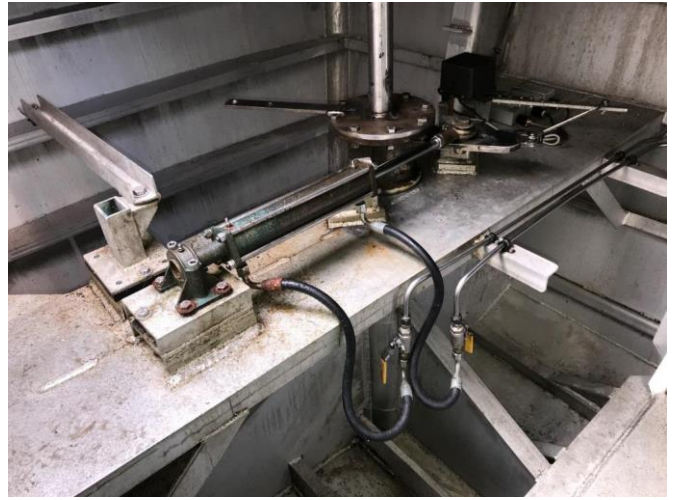
Photo # 56 – Comp. # 6 - Steering arrange. at port tiller-head
