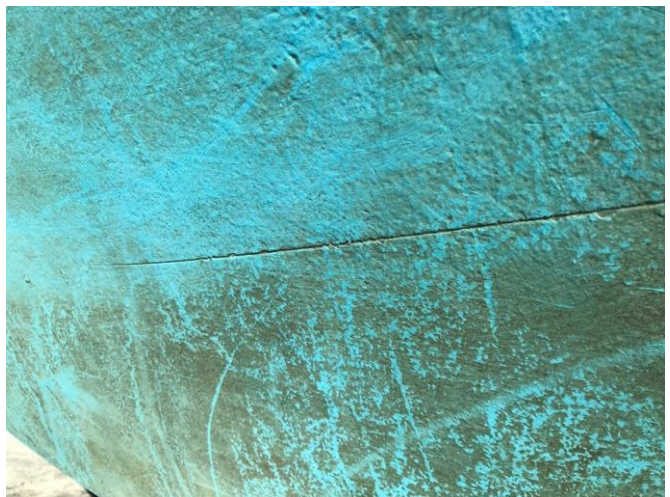
Photo # 2 – Bow hull (port side) with scrape indentation
