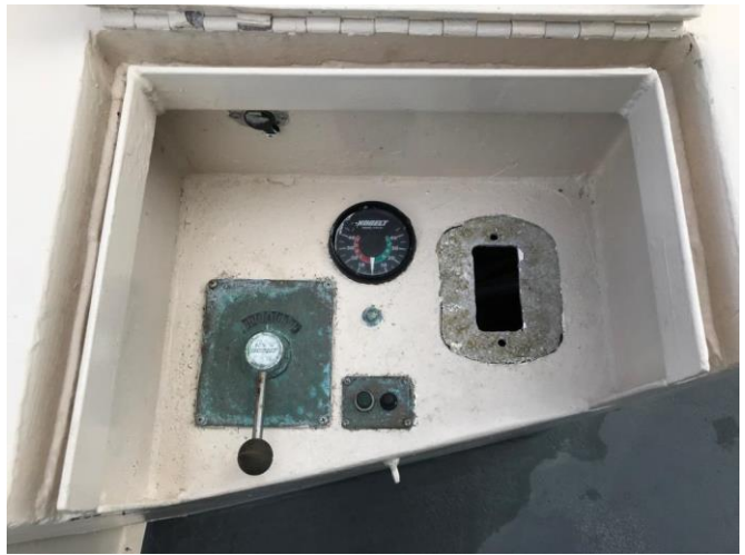
Photo # 34 – (P) Wing steering station with missing throttle control
