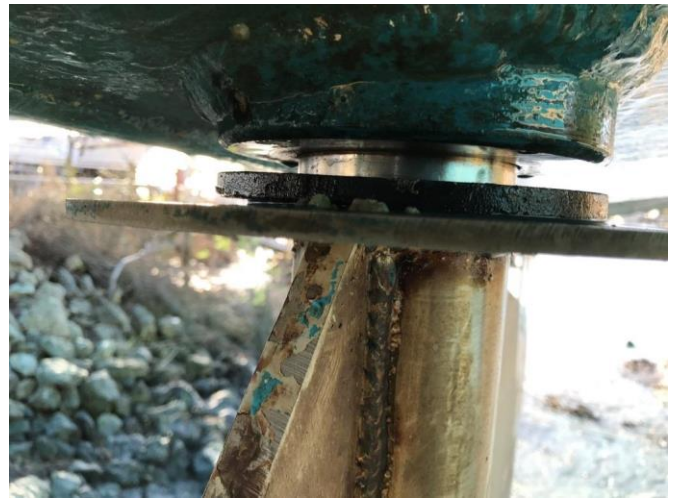
Photo # 12 – Typical condition of rudder bushing
