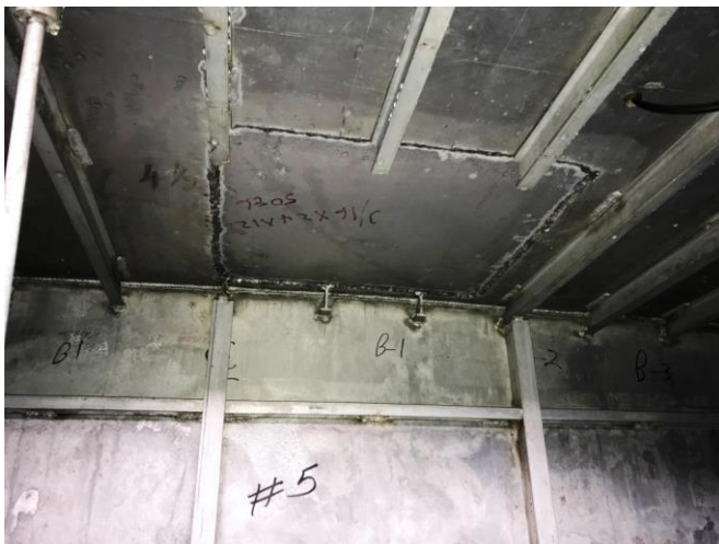
Photo # 35 – Fore peak deck insert with missing structure
