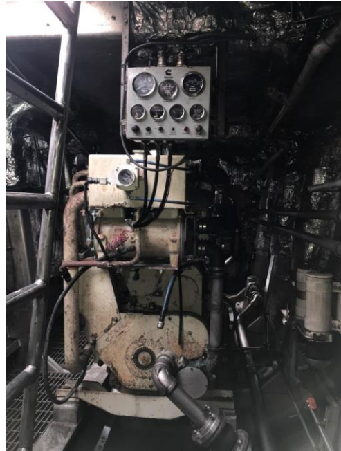
Photo # 46 – Comp. # 4 – 700 HP Main engine
