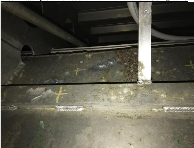
Photo # 59 – Comp. # 6S – Clad welding repairs to hull
