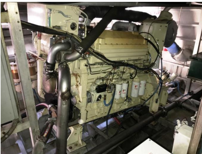
Photo # 41 – Comp. # 4 – Port side main engine – 640 HP
