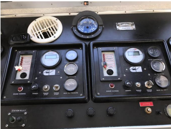
Photo # 41 – Cummins engine control panels at helm
