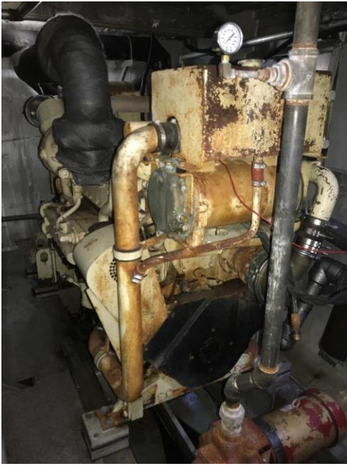
Photo # 47 – Comp. # 5 – Cummins 640 HP Main Engine
