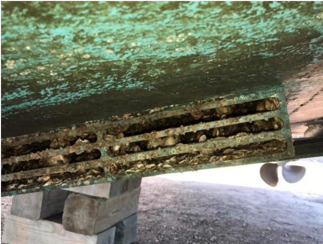
Photo # 9 – Main sea chest intake screen with heavy fouling
