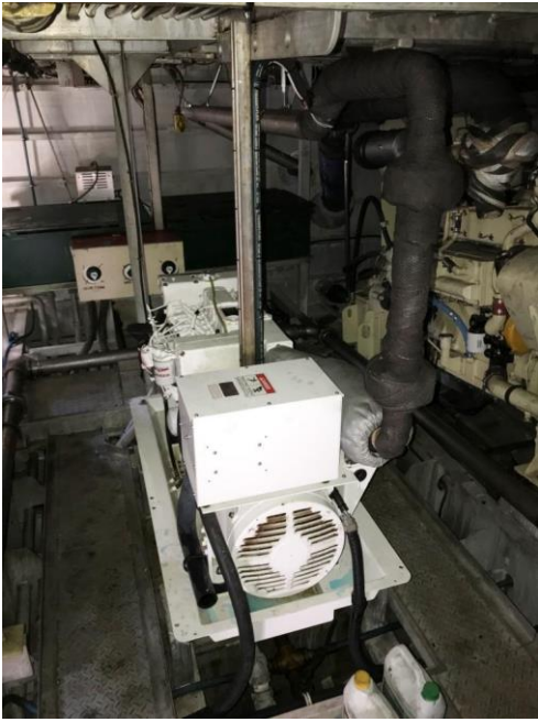
Photo # 43 – Comp. # 4 – Single gen/set – 30 kW
