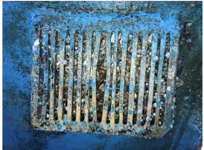
Photo # 6 – Port side main engine sea chest heavy fouling
