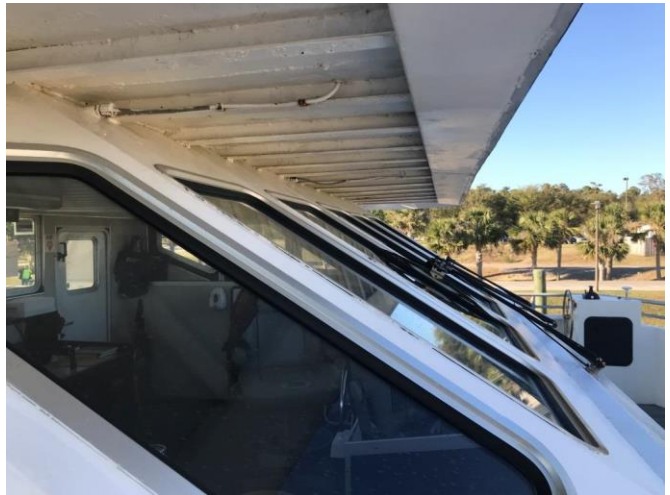
Photo # 34 – Forward bulkhead of pilot house with visor & windshield wipers
