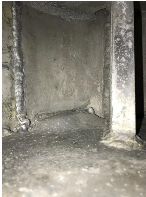
Photo # 16 – View of port bow damage from inside the fore peak
