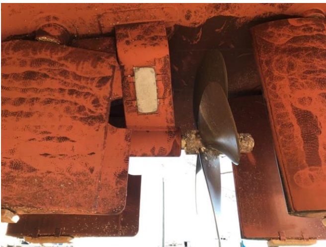
Photo # 7 – Stbd. tail shaft, prop, and rudders
