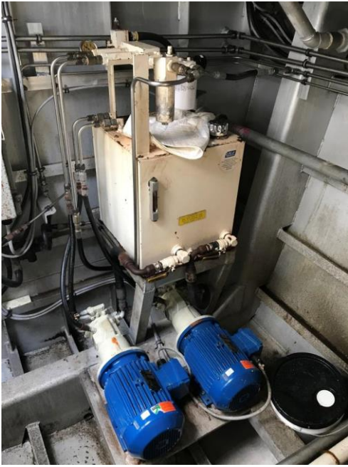
Photo # 55 – Comp. # 5 – Hydraulic steering system
