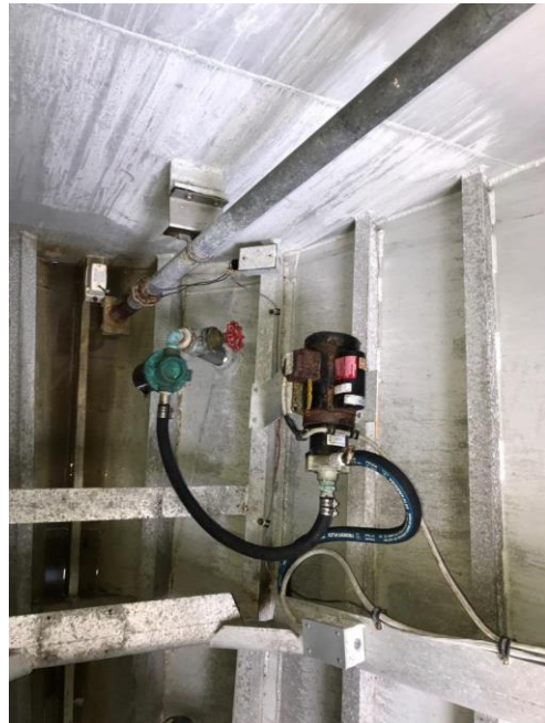
Photo # 42 – Comp. # 2 – Cooling pump sea chest & pump for fwd. HVAC, bilge suction, and level alarm
