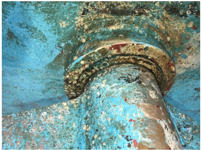
Photo # 12 – Typical condition of rudder bushing
