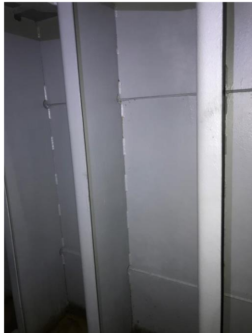
Photo # 28 – Sternlog construction with 1” x 18” PL top & bottom and vertical 15” x 3” x 5/16” Flg. PL stiffeners.
