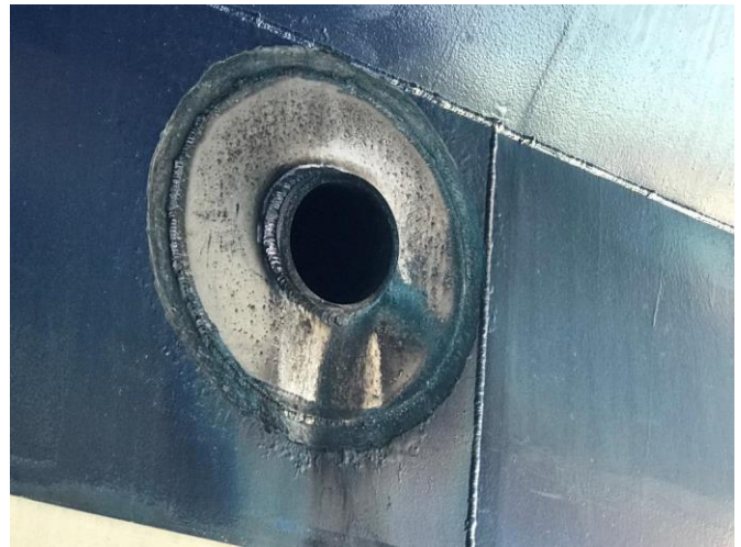
Photo # 10 – Starboard side main engine exhaust w/ reinforcement ring
