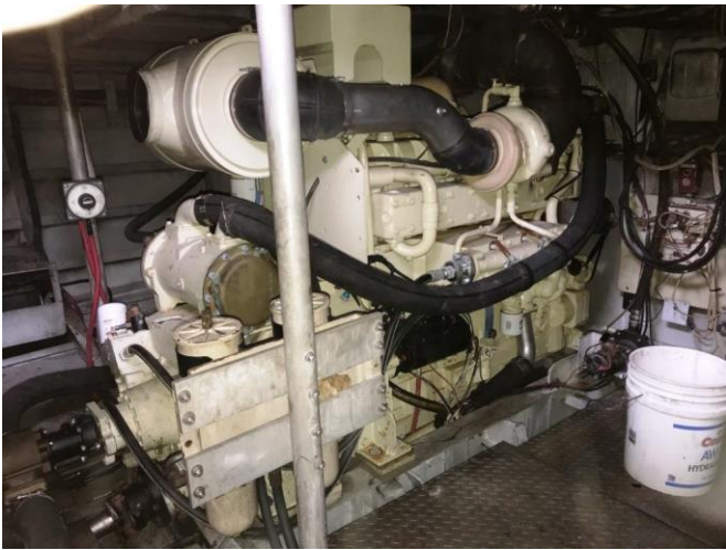
Photo # 31 – Comp. # 4 - Port main engine – 640 HP
