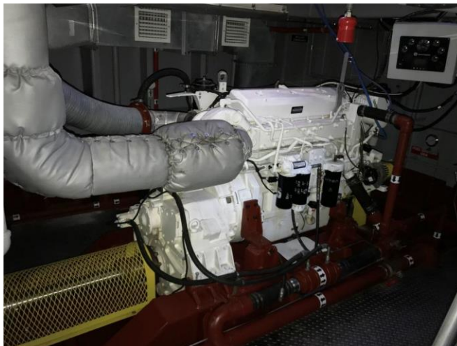
Photo # 26 – Port main engine – John Deere 425 HP
