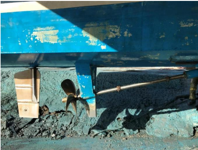
Photo # 5 – Starboard side tail shaft, prop, and rudder
