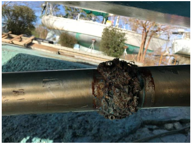
Photo # 14 – Wasted anode condition on propeller shaft
