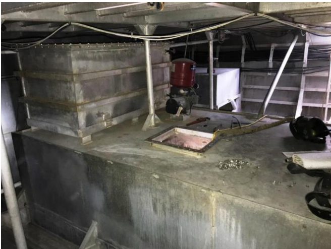
Photo # 29 – Compartment # 3 – looking to port showing main fuel tank & fresh water tank atop
