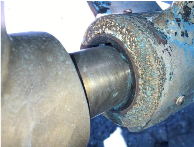
Photo # 11 – Typical condition of cutlass bearing at ‘V-strut’
