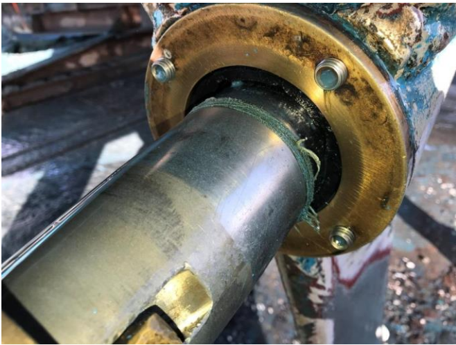
Photo # 13 – Typ. Condition of cutlass bearing at ‘V-strut’
