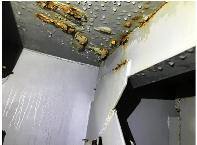
Photo # 18 – Typical condition of overhead in the fwd. rake.
