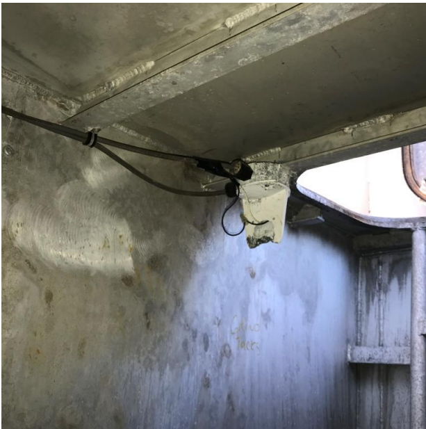
Photo # 45 – Comp. # 3P – Broken lighting fixture
