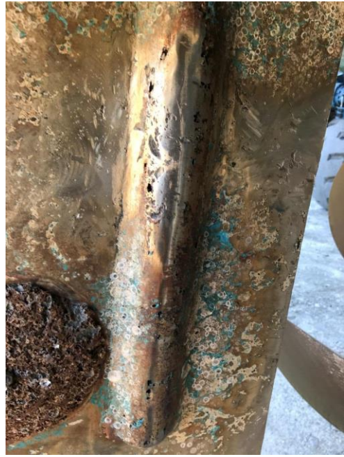
Photo # 8 – Port side rudder with 'pitting'
