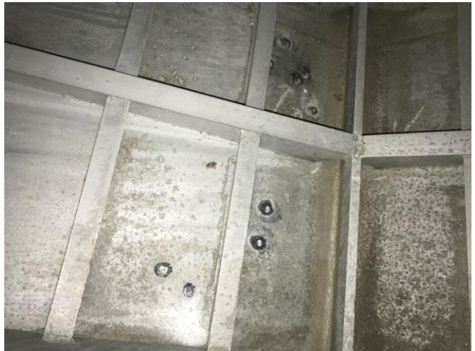
Photo # 40 – Comp. # 3 – clad welding on bottom hull
