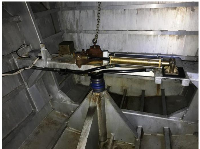
Photo # 58 – Comp. # 7P - Steering arrange. at port tiller-head
