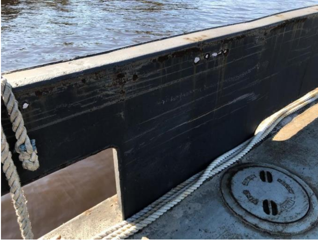
Photo # 7 – Typical wastage at port side bulwark
