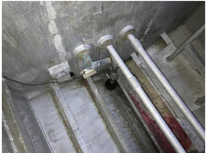
Photo # 46 – Comp. # 3P - Bilge suction piping & bilge alarm
