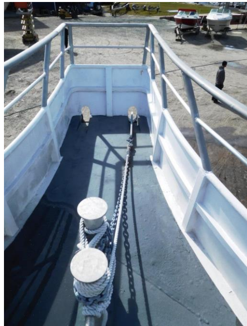
Photo # 20 – Bow sprit with anchor arrangement
