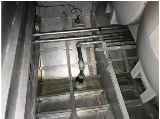
Photo # 38 – Comp. # 3 – bilge alarm, suction, & transducer
