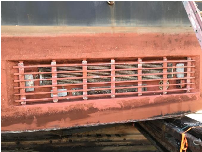
Photo # 5 – Port side main engine grid cooler and sea chests
